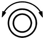
Turn to the right to brighten the picture. (The normal setting for this knob is at the center, click-stop position.)
