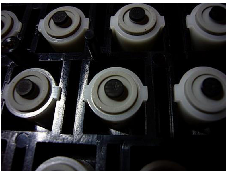
BELOW: a close-up image of the carbon-faced plungers which strike the PCB switches NOTE: my defective 'E' key is in the centre of the picture - notice the dirt on it ?
