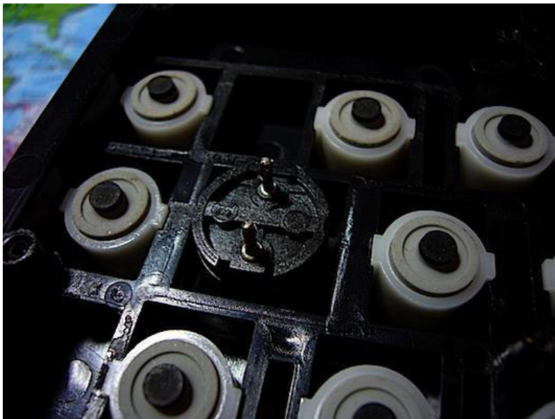
BELOW: Plungers that strike the PCB switches when a key is pressed (notice the solder posts in the pic centre)
