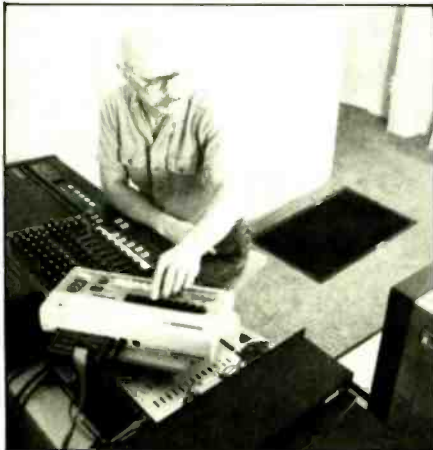
The Synchronous Technology SMPL Chase Lock system (seen with reviewer Bob Hodas above) comprises a modified Commodore VIC-20 PC running custom software (right) connected via an interface card to an external transport, timecode, sync and MIDI controller (below).
