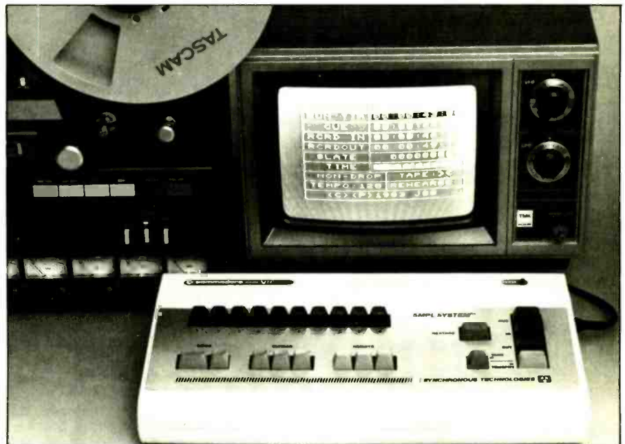
The Synchronous Technology SMPL Chase Lock system (seen with reviewer Bob Hodas above) comprises a modified Commodore VIC-20 PC running custom software (right) connected via an interface card to an external transport, timecode, sync and MIDI controller (below).
